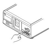
**3** Turn the JOG dial until you find the disc slot where you want to insert a disc, while checking the disc number (written beside every slot and also indicated in the display).
