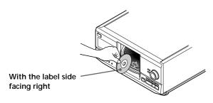
After inserting the disc, you can input the original disc titles instead of the disc numbers (see "Labeling Discs" on page 18) to locate it easily when you start playing.
